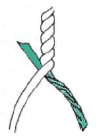
Figure 2: The new strand was twined in with the original.
